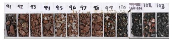
Photo 1: NMWBRC22-605 90-103m – Hematite + Albite + Quartz altered Quartz Porphyry (10m @ 5.80g/t Au - within 13m @ 4.53g/t Au from 90m)
