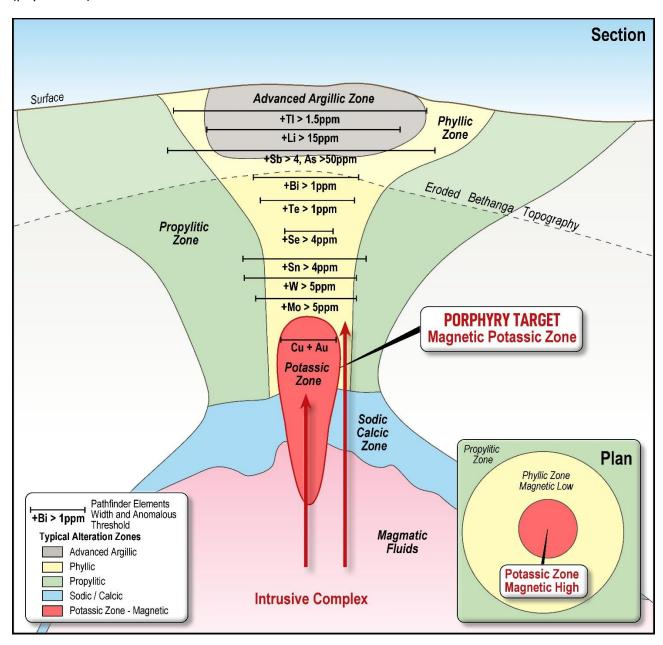
Figure 9: Schematic diagram showing the geophysical signatures of the potassic and phyllic zones.
