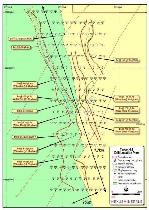
Figure 5: Wallbrook Regional Target 4.1 Aircore Drill results over Geology
