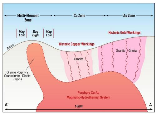
Figure 13: Geological Cross Section A-A' Exploration Model
