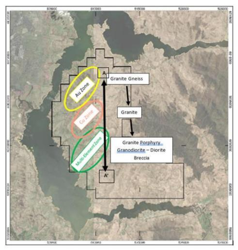
Figure 12: Geological Plan Exploration Model over Topography (Cross section A-A' see below figure 7)
