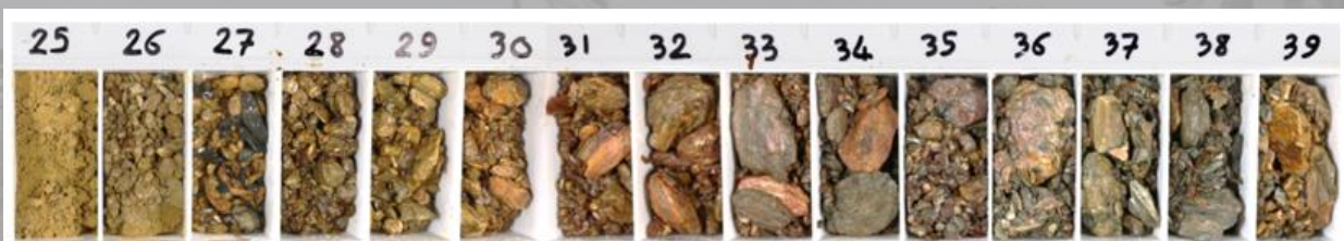
Photo 2: NMWBAC24-651: 4m @ 4.02 g/t Au (from 28m) within 15m @1.30g/t Au (from 24m)
