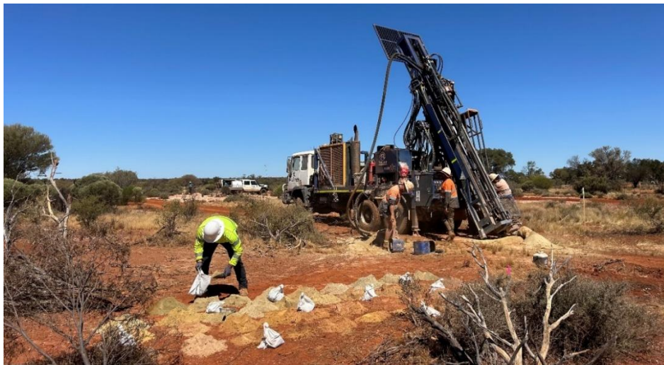
Photo 1: Aircore Rig at Wallbrook Gold Project
