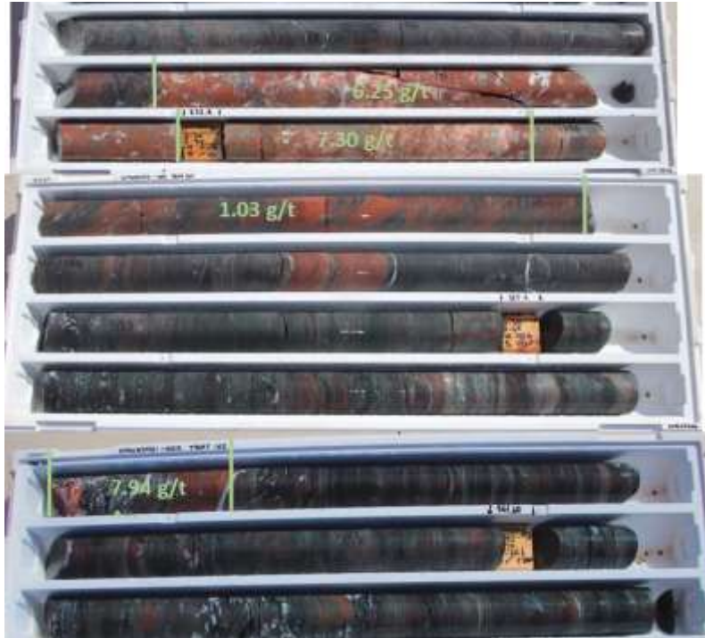
Photo 1: DDH21-2 551.53m – 553.95m 2.42m @ 4.28g/t Au and 0.25m @ 7.94g/t Au within 9.77m @ 1.35g/t Au, from 550.53m Mineralisation hosted in silicified quartz porphyry unit with extensive alteration and stockwork veining
