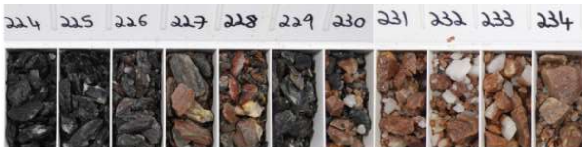
Photo 1: Hole #178 10m @ 5.49g/t Au (from 224m) - Incl. 4m @ 12.49g/t Au (from 228m)
