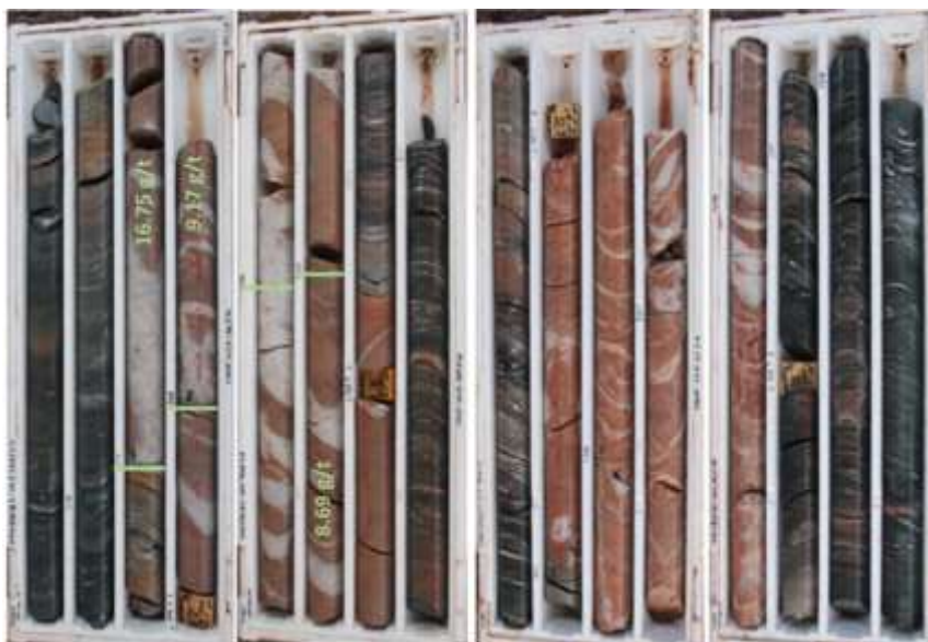
Photo 3: Crusader DDH21-1 159m – 168m. 3m @ 11.54g/t Au, within 9m @ 4.49g/t Au, from 159m Mineralisation hosted in silicified quartz porphyry unit with extensive alteration and stockwork veining
