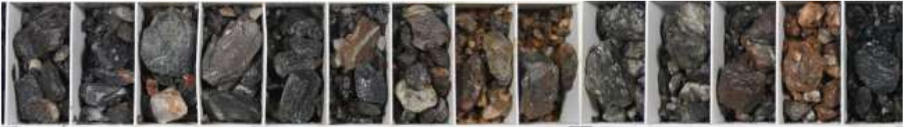
Photo 1: Hole #176 14m @ 8.80g/t Au (from 141m) - Incl. 3m @ 21.59g/t Au (from 149m) Mineralisation showing extensive alteration and stockwork veining
