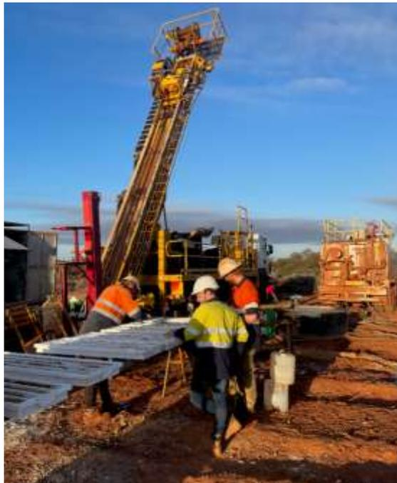
Photo 1: Diamond drill rig at Crusader Gold Prospect
