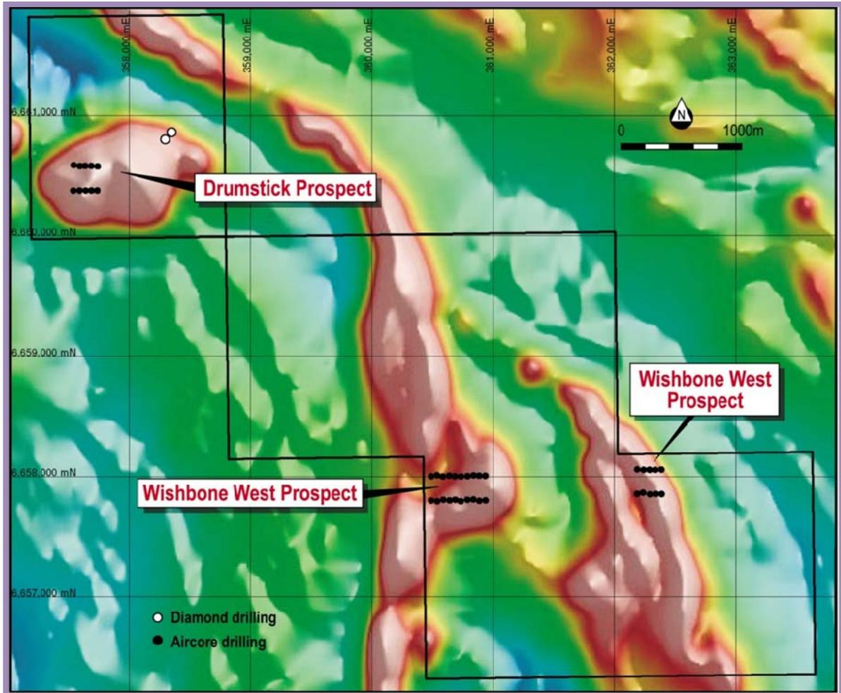
Figure 2: Mulgarrie Project showing magnetics and Hemisphere drilling
